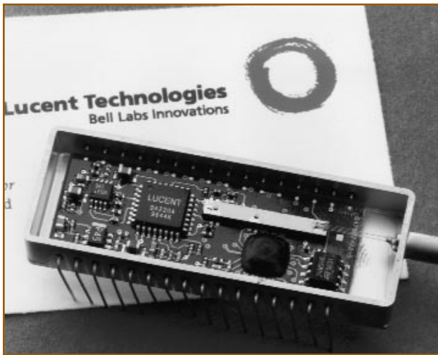
Figure 15. Prototype bidirectional transceiver for low-cost fiber-to-the-home applications integrating several functions on a single silicon wafer.
